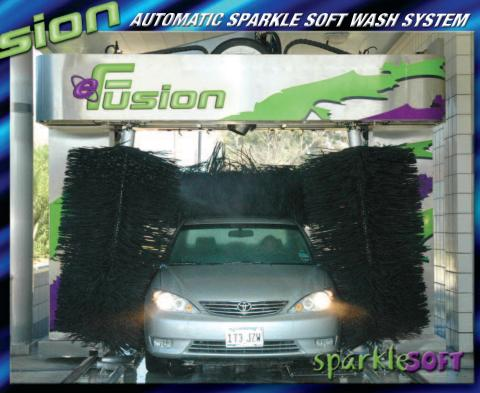
The eFusion is designed to efectively clean a vehicle using our unique SparkleSoft foam brushes. SparkleSoft is a strong, hushed and delicate product that glides over the vehicle's surface, enhancing gloss and luster.
