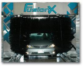
vehicle. Each brush uses an amp sensing technique to stay in constant contact with the vehicle and with just the right amount of cleaning pressure to ensure a clean vehicle.
