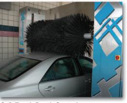
Soft Touch Brush Controls The system uses a Multi-Axis Coordinated Brush Motion Control to adjust the top and side brushes to the exact contour of every
