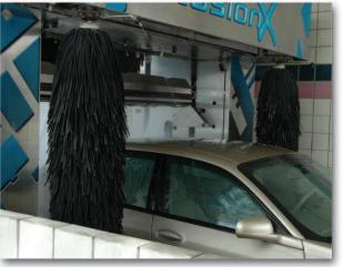
Maximum cleaning in a touchfree automatic depends on quality hot presoak and good high pressure scrubbing action. Moving the nozzles closer to the vehicle during the high pressure passes produces consistent and effective cleaning power.
