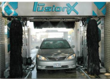
**Spot Free Rinse** The final rinse is delivered with a distinctive cone pattern spray on top and wide angle nozzles on the sides for a thorough spot free rinse.
