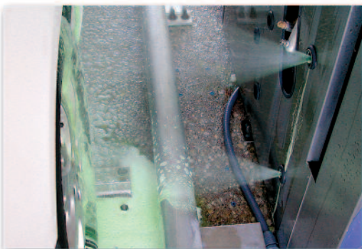
Above: On-board tire cleaning applications. Below: Zero degree oscillating nozzles deliver an extra blast of cleaning power.
