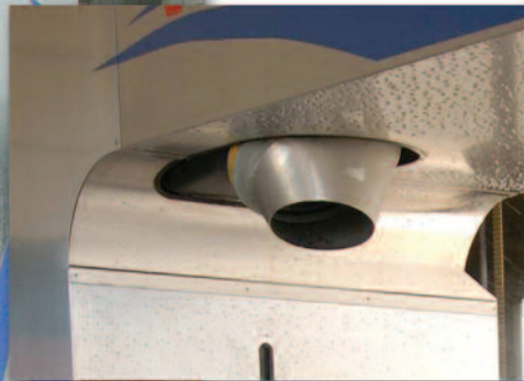
Side blowers can be easily adjusted for maximum performance.
