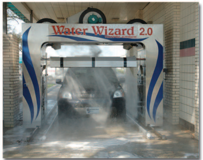
The scrubbing action oscillating nozzles sweep back and forth over the entire vehicle as the wash gantry passes over the vehicle.
