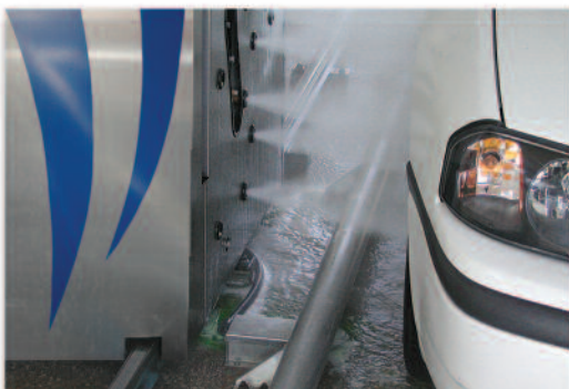
Above: On-board tire cleaning applications. Below: Zero degree oscillating nozzles deliver an extra blast of cleaning power.
