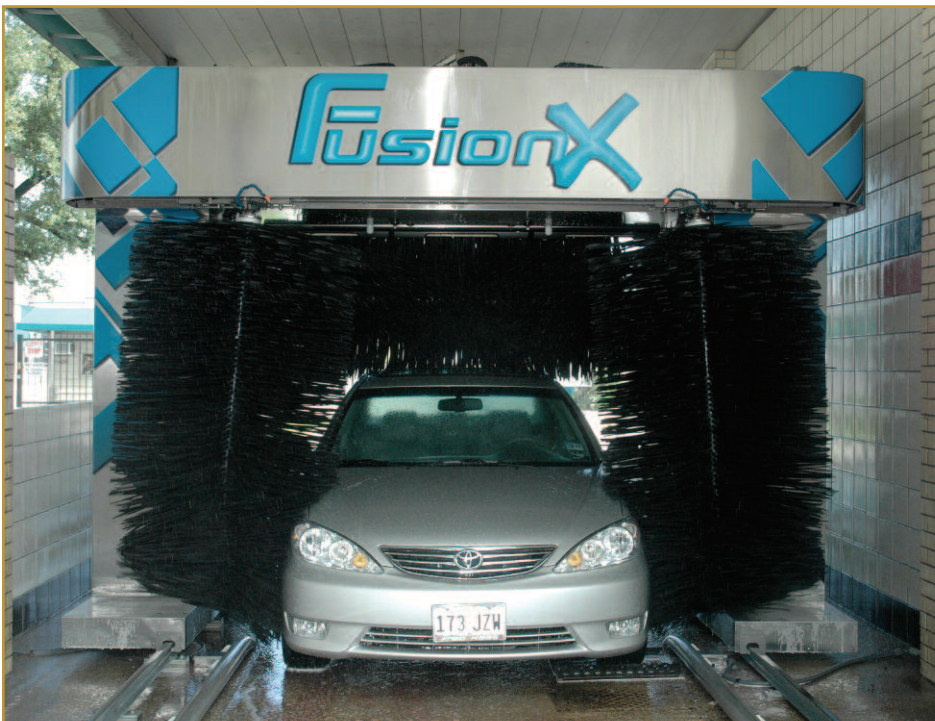
FusionX is a combination wash where the customer can choose between touchless and friction/brushes.
